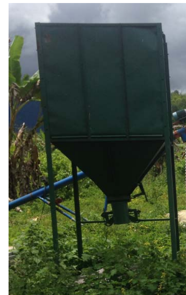
Hoppers with baggers
